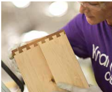
Sturdy dovetail construction
